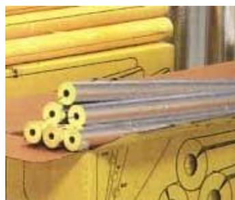
**Moy Isover Foil pipe insulation** with a factory applied reinforced aluminium foil 'Class-O' facing incorporating a self adhesive overlap, is suitable for use on pipes operating at below ambient temperatures.
